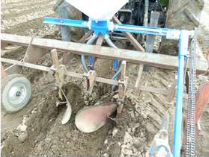
Horstine applicator, modified to place fertilizer in the furrow with the asparagus crowns © ADAS
